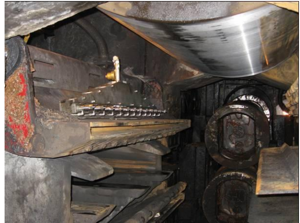
Figure 8: Pure oil lubrication implemented at ArcelorMittal Dunkerque
