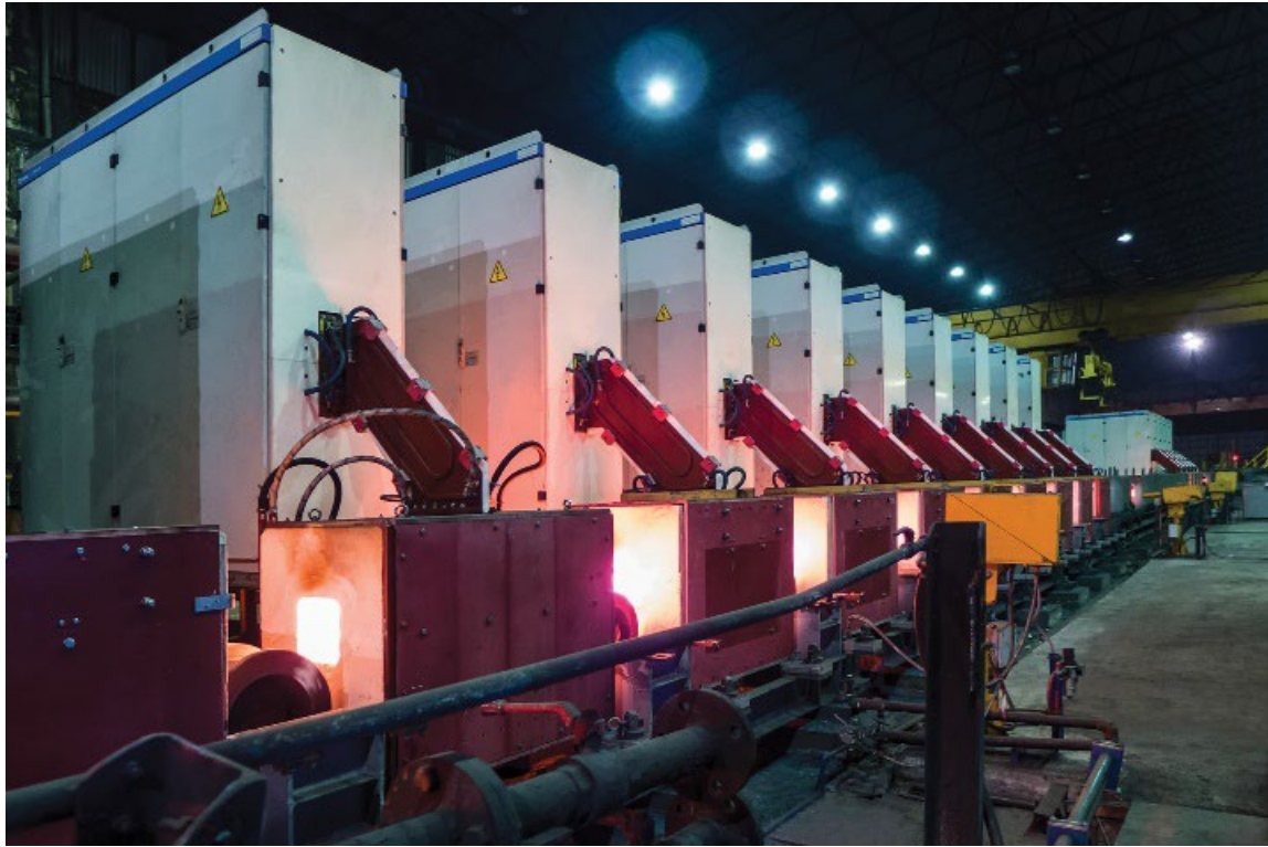
Figure 2 : Induction heating for billets [4].
